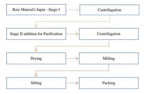
The process flow chart of other products manufactured by the Company, on demand basis, is given below. The quantity produced completely depends on the orders received.
